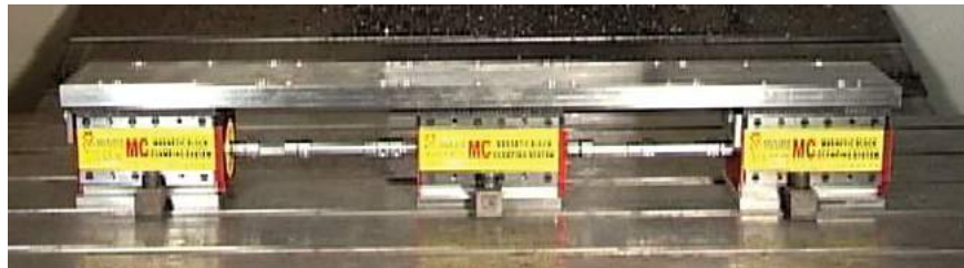
Switch-connect ECB vises to turn ON/OFF simultaneously
