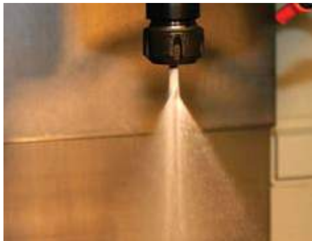
Removing the o-ring creates a CoolBLAST coolant effect.
