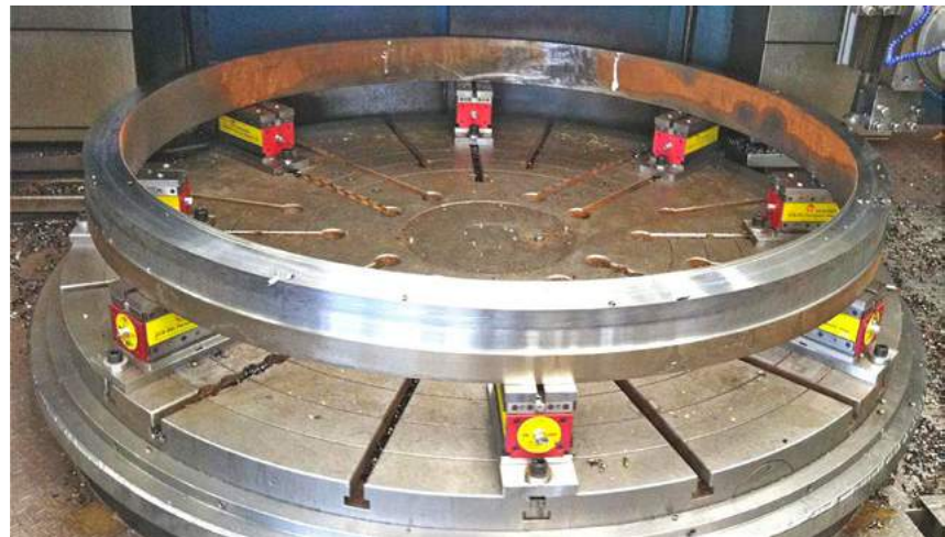
ECB magnetic vises are easy to setup for vertical turning. Machine both O.D. and I.D.
