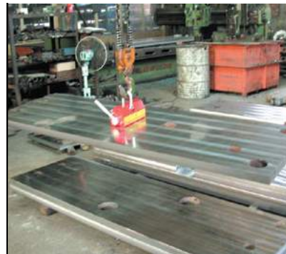
Locate magnet at balance point for lifting.
