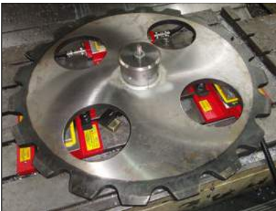
Large tooth sprocket being machined
