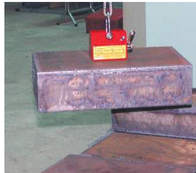
Center magnet on most workpieces to lift.
