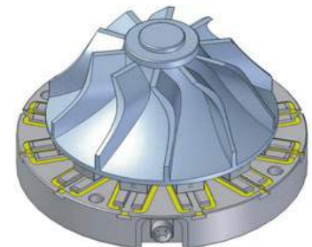
5-axis turbine blade machining
