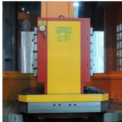
2-sided EEPM on palletized system
