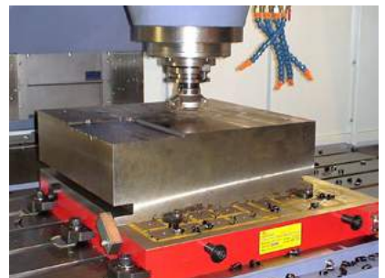
Face milling on workpiece with work-stops installed
