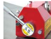
Lever in the "ON" position engages safety lock.
