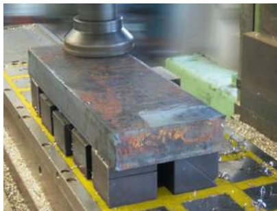
Use spring-loaded blocks for warped stock
