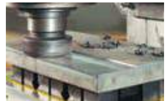
Milling warped stock with induction blocks
