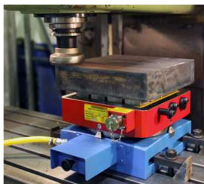
Use induction blocks to machine full 5 sides freely
