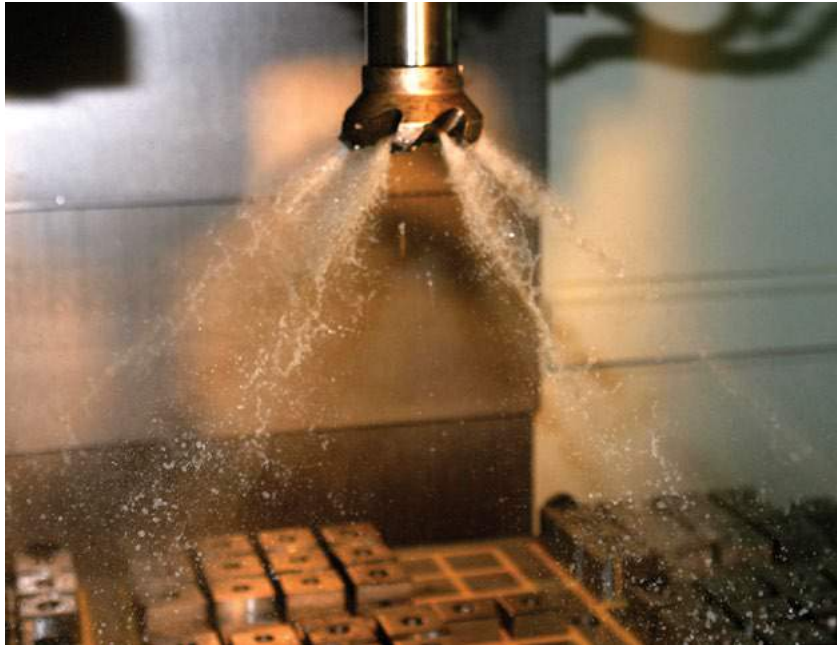
CoolBLAST arbor screw provides coolant path.
